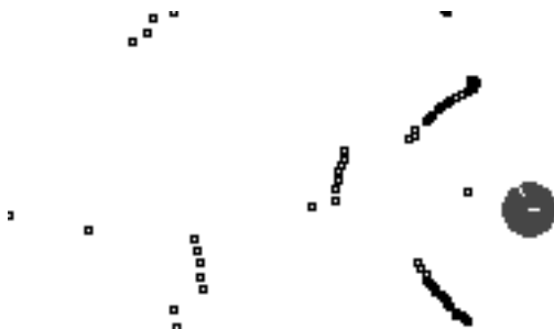
Figure 6.4 Sonar Scan on a Corner
